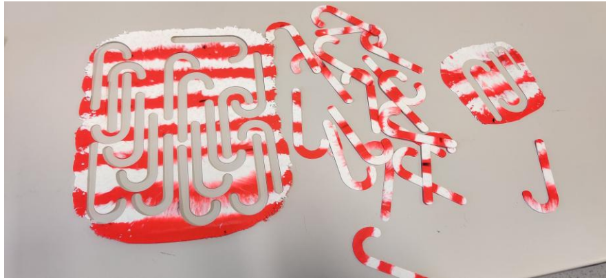
Figure 4 - 3D printer filament recycled into sheet material for the laser cutter
