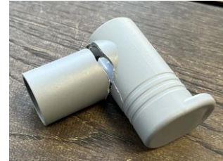
Figure 3 - Damaged clothes rail mount
